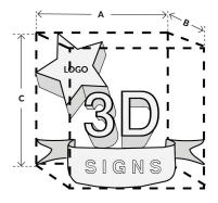
Sign area is computed using the smallest rectangular prism that will encompass the entire sign. (2(A x C) +2(B x C))
