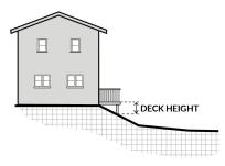
FIGURE 18.02.030.C.2: MEASURING HEIGHT OF DECKS
